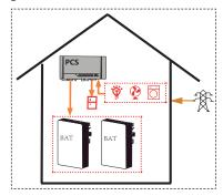
Battery can be charged by grid. Users are suggested to store energy from grid to battery when electricity price is relatively lower.
