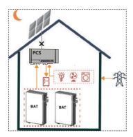
Battery powers loads at nighttime when there is no PV. If battery energy is insufficient, it can enpower loads together with grid.
