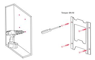
Step 3. Fix battery on bracket.
